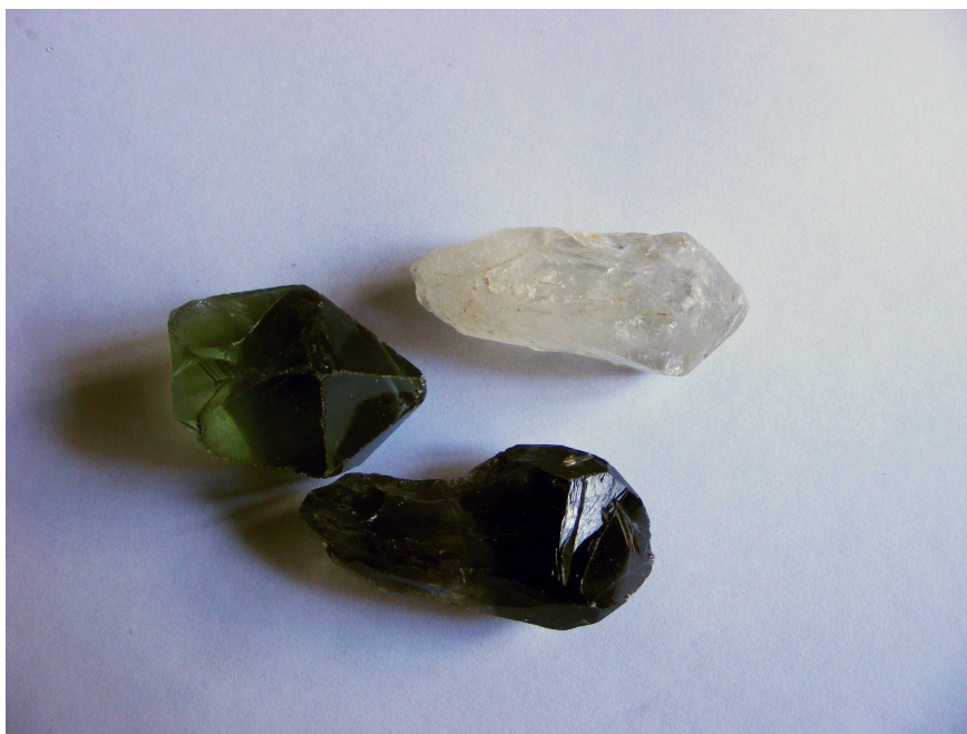
Figure 2. Hydrothermal quartz , natural crystal without color, green colored crystal produced by irradiation to 450 kGy and a smoky green color produced by the same dose.
