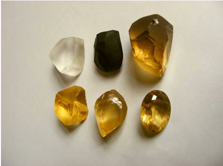
Figure 3. Quartz crystals from pegmatite, Itamarandiba, above from left to right, colorless, blackened by irradiation to 1000 kGy, and heated at 260 degree for 1, 2 and 3 hours. Shown also cut gemstone.
