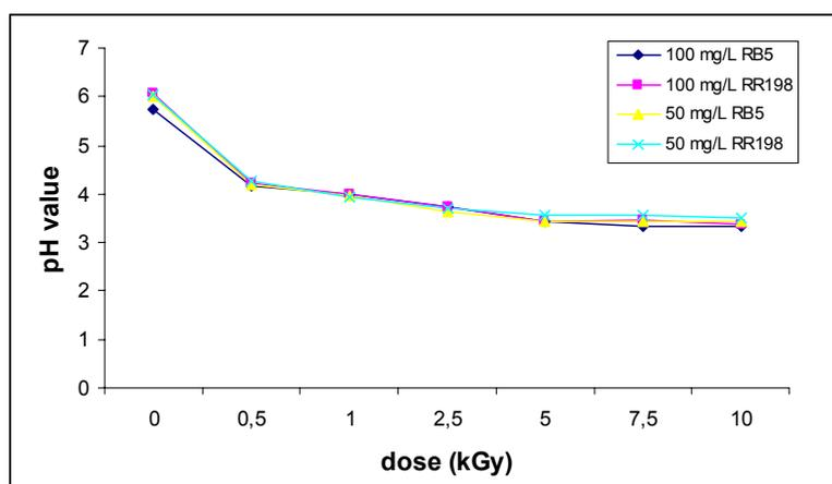
**Figure 4. The change of pH value under electron beam irradiation of RB5 and RR198 solution.**
