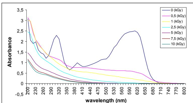
**Figure 2. Absorbance spectra of RB5 ( $100 \text{ mg L}^{-1}$ ) versus radiation doses (kGy).**
