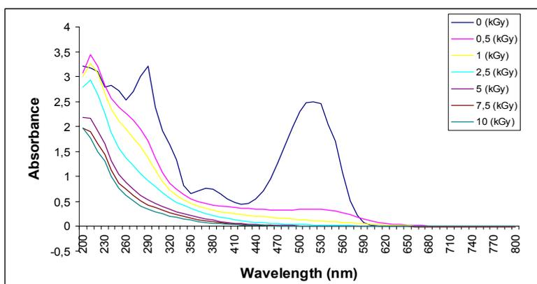
**Figure 3. Absorbance spectra of RR198 ( $100 \text{ mg L}^{-1}$ ) versus radiation doses (kGy).**
