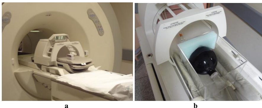
Fig. 4. Experimental set up for MRI images acquisition of the FXG cuvettes (a) and phantom (b)
