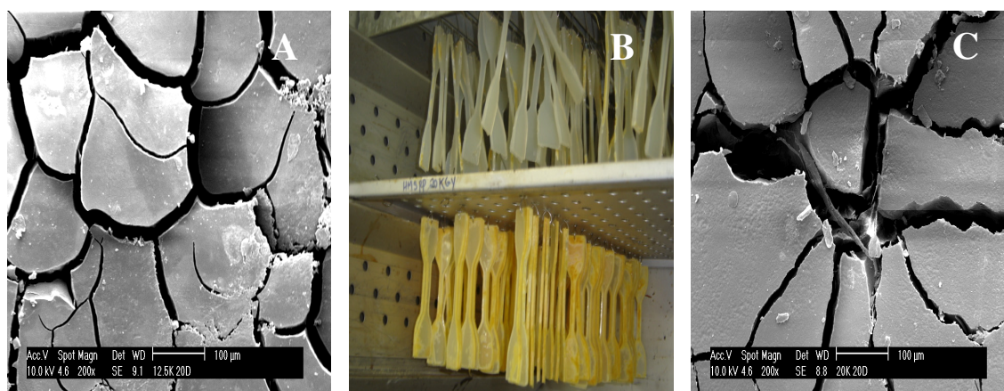
Figure 1 -: (A) Scanning Electron Microscopy (SEM), HMS-PP 12.5 kGy, 100 µm, (B) Dumbbell samples degradation in Stove, (C) SEM, HMS-PP 20 kGy, 100 µm.
