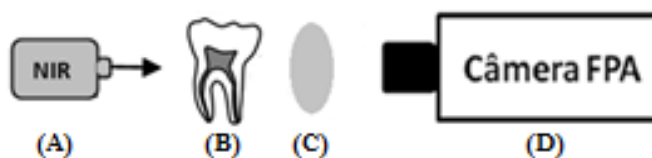
Figure 1 - Experimental arrangement: A) NIR source, B) Samples, C) Optical filters and D) FPA Camera.
