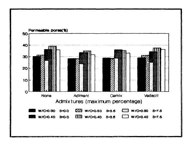
Figure 3 - Total volumetric percentage of permeable pores in cement pastes for W/C = 0.3 and 0.4, different salt contents and admixtures types
