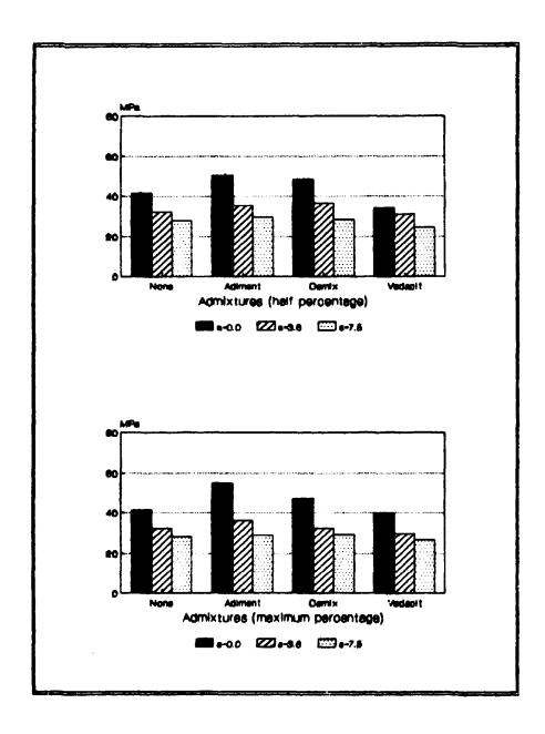
Figure 6 - Compressive strength of cement pastes with W/C = 0.40, different NaNO<sub>3</sub> contents and admixtures
