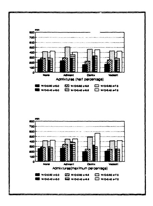
Figure 1 - Initial setting time of cement pastes for different W/C ratios, NaNO: contents and admixtures types
