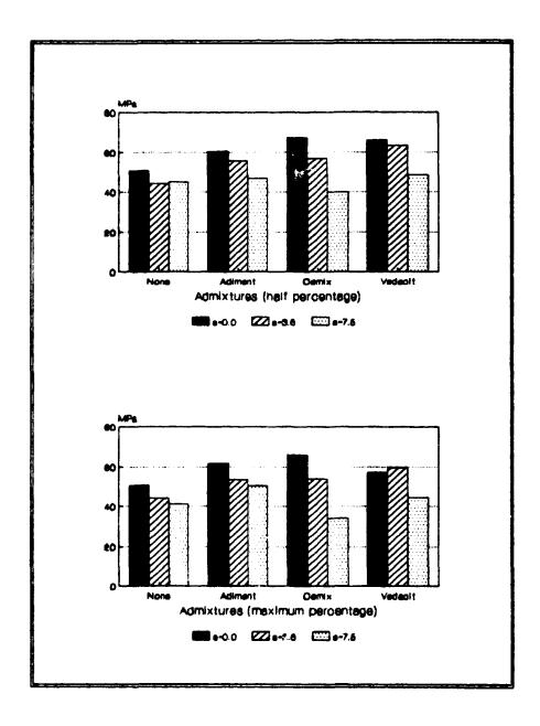
Figure 5 - Compressive strength of cement pastes with W/C = 0.30, different NaNOs contents and admixtures
