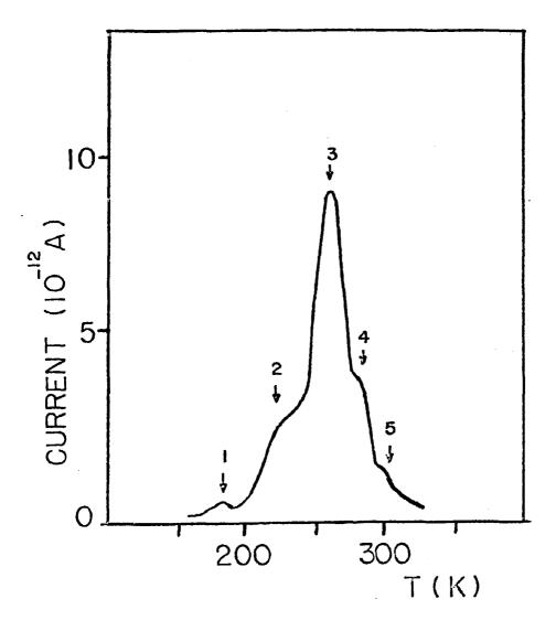
Figure 1 = Thermally Stimulated Depolarization Current spectrum of polycrystalline Thorium Dioxide; polarization conditions:  $T_p = RT$ ,  $t_p = 120$  s,  $E_p = 5000$  V/cm; heating rate: 4 deg/min
