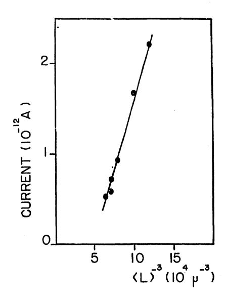
Figure 4 — Correlation between the induced polarization (plotted here as the amplitude of peak 3 in the TSDC spectrum) and the average crystallite size of polycrystalline ThO<sub>2</sub>
