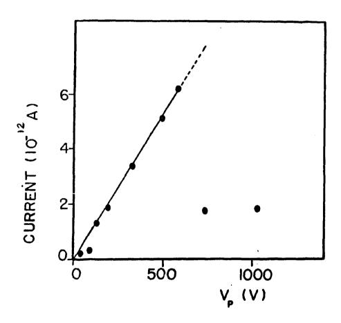
Figure 2 — Dependence of peek 3 maximum amplitude on the polarizing voltage for ThO<sub>3</sub> polycrystelline samples
