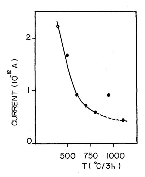
Figure 3 — Dependence of peak 3 maximum amplitude of TSDC spectrum of polycrystalline ThO<sub>3</sub> on the sintering temperature; sintering atmosphere: air
