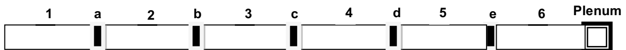
1, 2, 3, 4, 5, 6: 36.5 cm (25 fuel pellets) divided in 4 segments each one of 91 mm (apart the first two meshes of 85 mm); a, b, c, d, e: 40 mm (stainless steel disk); Plenum: 140 mm
