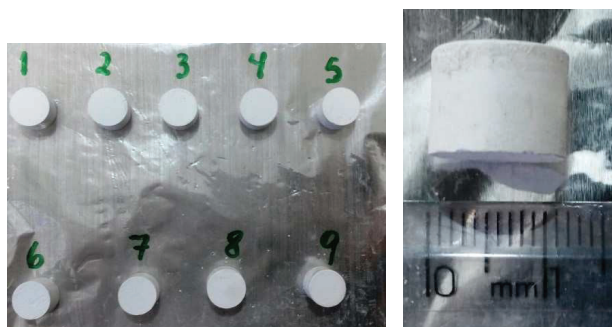
Fig. 1 Uniaxial compacted pellets with pure ThO 2 powder.
