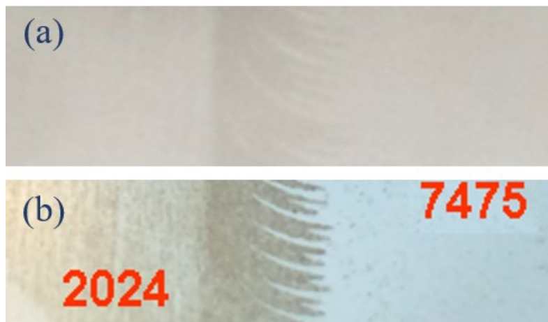
Figure 7. Macrographs of the dissimilar alloys AA2024-T3 and AA7475-T761 welded by FSW (a) prior to immersion and (b) after 24 hours of immersion in 0.1 \text{ mol L}^{-1} \text{ Na}_2\text{SO}_4 solution
