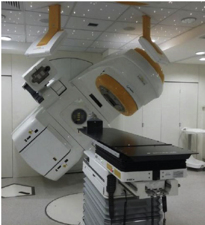
Fig. 4. 'STEEV' phantom positioned over the couch of treatment in the VARIAN NOVALIS TX linear accelerator of HSL.
