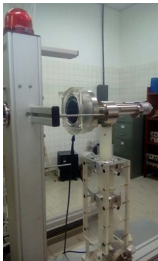
Fig. 2. Extrapolation chamber entrance window covered by a Hostaphan absorbing sheet.
