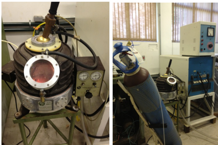
Fig. 1. Pictures of the furnace-gas-rectifier ensemble used to produce Zr1Nb alloys.
