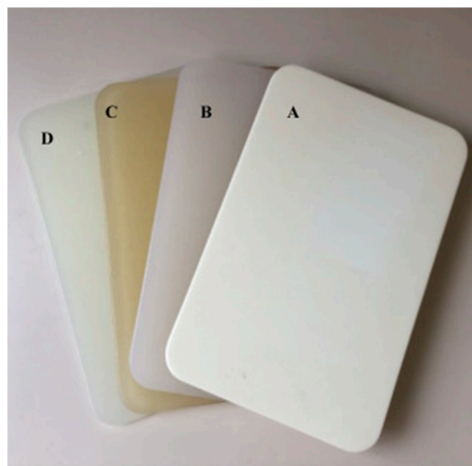
Fig. 1. Tissue equivalent samples produced A, B C and D resin-based materials.
