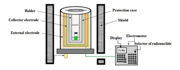
Figure 1: Representation of a well-type activity measuring instrument.
