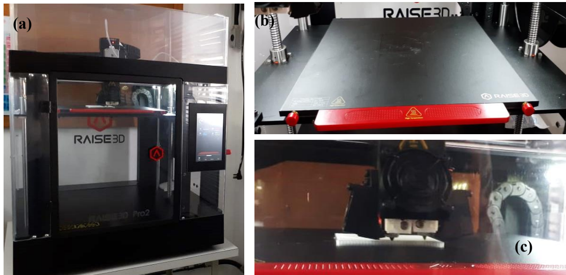
Figure 1. RAISE 3D PRO2 printer from IPEN (a) general view (b) detail on heated bed (c) detail on extruder nozzles
