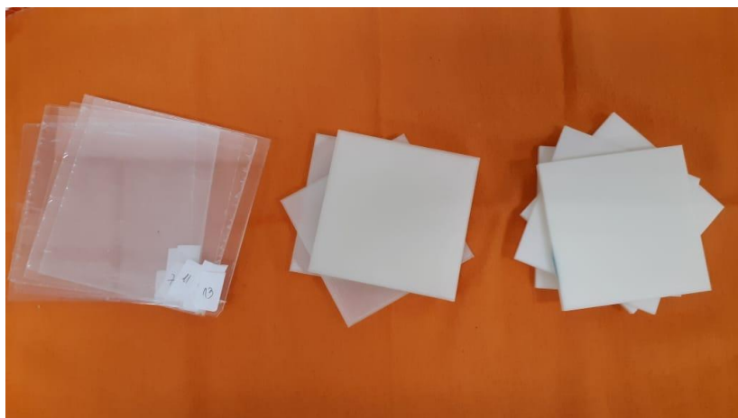
Figure 2. PMMA, PLA and ABS phantom plates used for radiation transmission measurements
