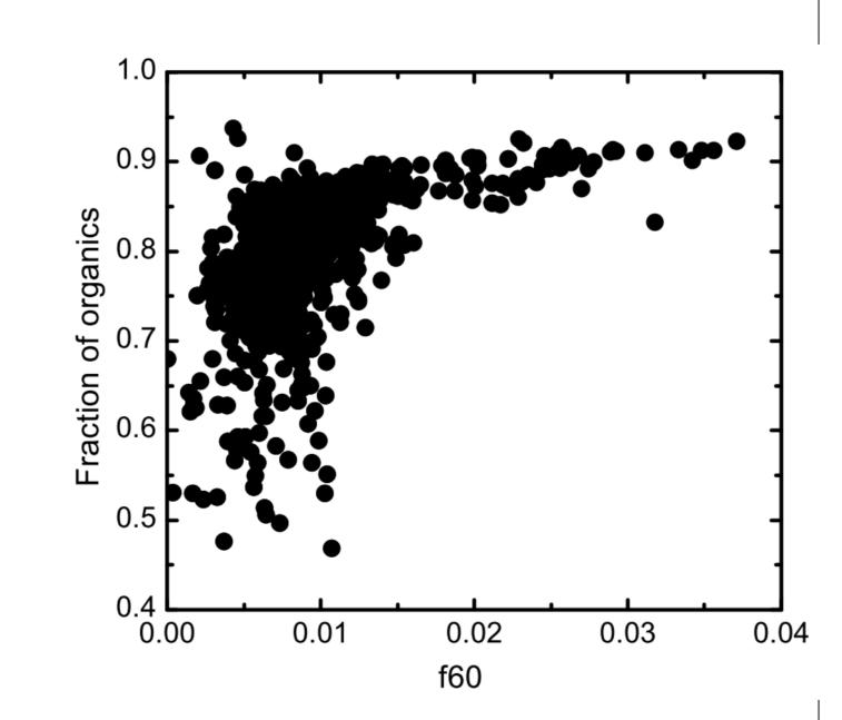
The biomass burning aerosol, studied using a Van Krevelen diagram, was observe to be processed by the change in the O:C ratio only, consistent with the replacement of a hydrogen with an alcohol group (-OH), for example. The parameter f60 is a biomass burning marker.
