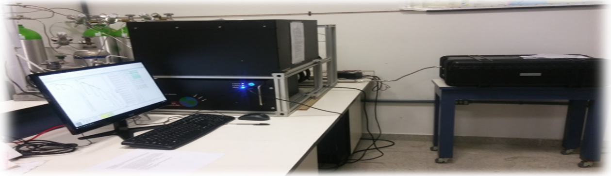
Figure 3. TILDAS-D CO 2 Analyser from Aerodyne Inc connected in PFP (version II, with 12 flasks)
