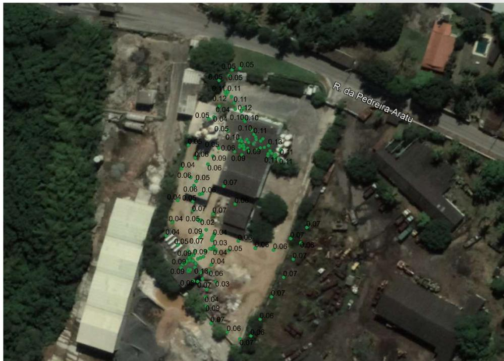
The radiometric survey of the working area was evaluated by using a Geiger-Muller. The mean exposition rate was  $0.07 \mu\text{Sv/h}$  ( $0.6 \text{ mSv/y}$ ).
