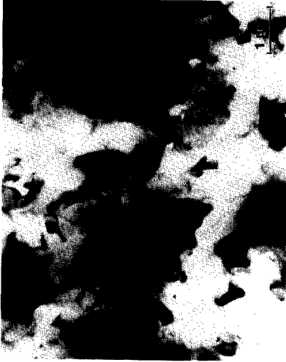
Fig. 7. TEM micrograph showing in the SNA side of the SNA/SNY + \text{ZrO}_2 couple. Pocket of \text{ZrO}_2 particles (dark) surrounded by \beta\text{-Si}_3\text{N}_4 and \text{Si}_2\text{N}_2\text{O} grains (BF image).
