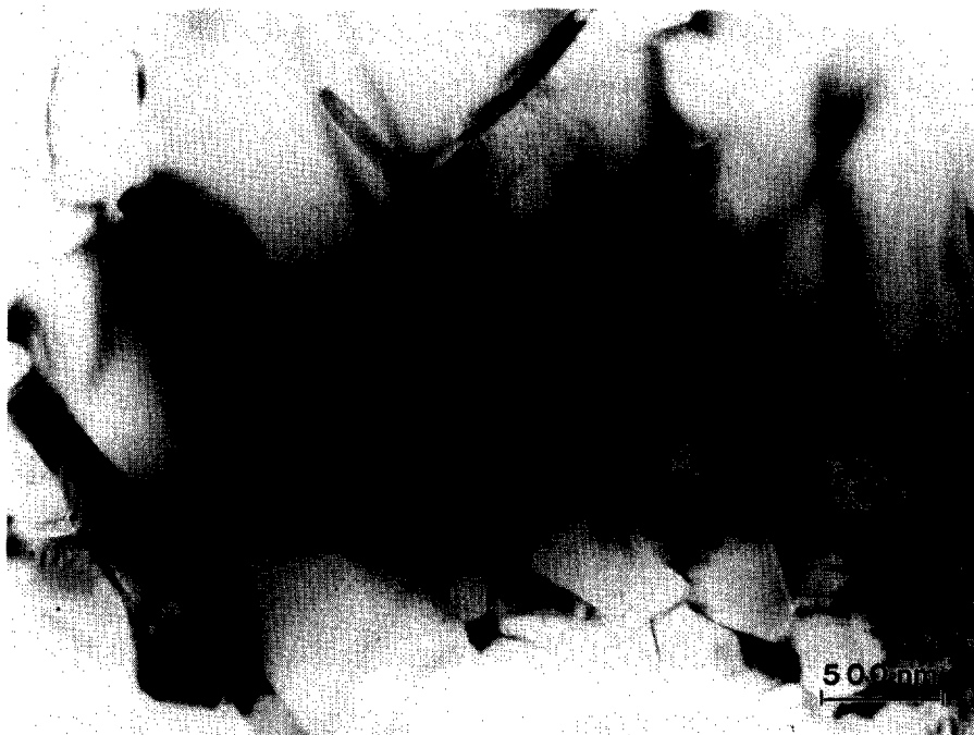
Fig. 11. BF image of a pocket of crystallized Zr_3Y_4O_{12} phase surrounding small \beta - Si_3N_4 grains in the SNY side of the SNA/SNY- ZrO_2 .
